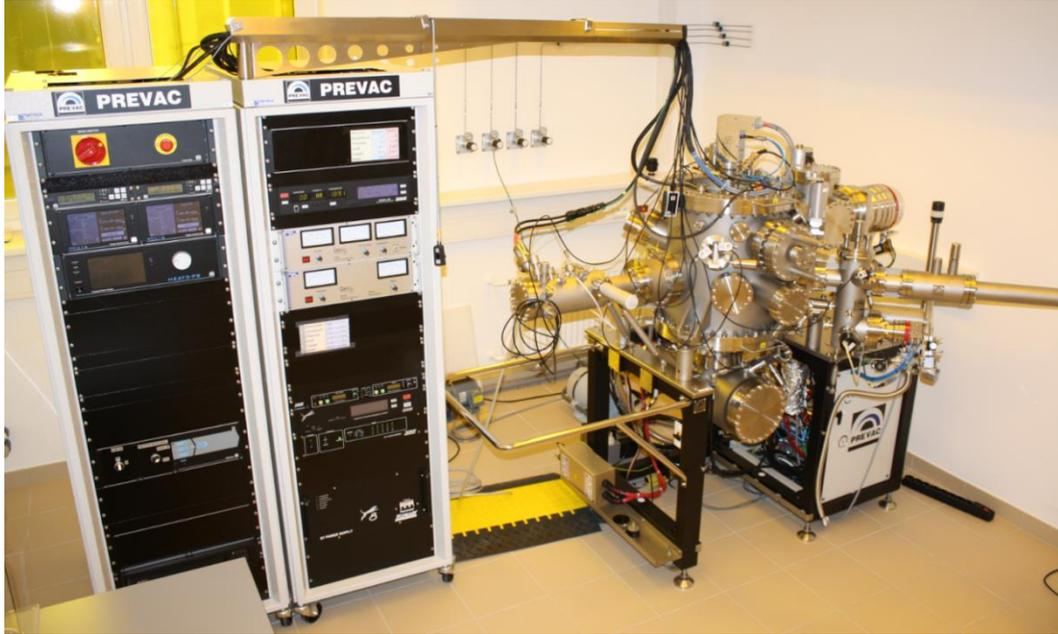
**Fig.21. Electron-beam evaporator with ion gun.** Base vacuum  $2 \cdot 10^{-9}$  mBar (without annealing). The system is compatible with multi-angle e-beam lithography.
