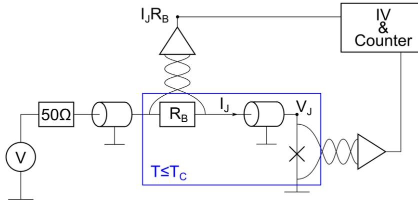
**Fig.5.** A simplified electrical circuit used in my laboratory to probe a junction with current pulses. It allows also to measure current-voltage (IV) characteristics of the junction ( $X$  in the figure). A counter (oscilloscope) records number of switching events observed as a voltage pulses  $V_J$  developing on the junction.  $R_B$  is a bias resistor for monitoring the current sent to the junction  $I_J$ .  $V$  stands for Arbitrary Waveform Generator (AWG) with  $50\Omega$  output.
