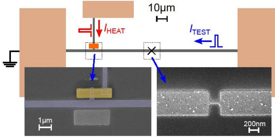
**Fig.12. Layout of the sample** for studying the dynamics of hot electron diffusion at milliKelvin temperatures. It consists of resistive copper island (SEM photo to the left) and a remote temperature sensor (aluminum nanowire). A short heating pulse  $I_{HEAT}$  creates hot electrons which start diffusing towards thermometer along superconducting nanowire. The test pulse  $I_{TEST}$  is launched with time delay and probes temperature of the bridge (**Fig.13**).
