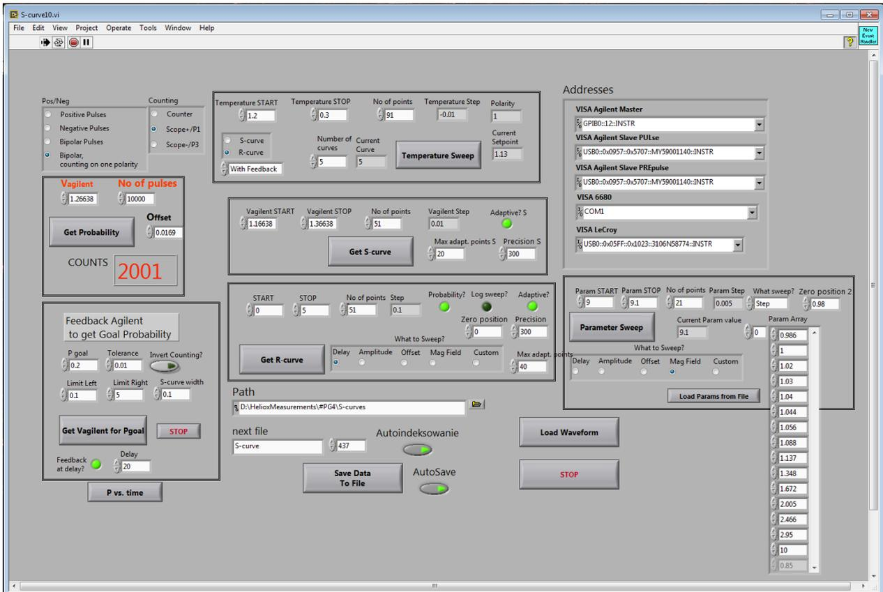
**Fig.23.** Front Panel of the **LabView acquisition program for performing switching measurements on Josephson junctions** developed over recent years by me. All data presented in publications **H1-H5** were acquired with that software being extended in time.
