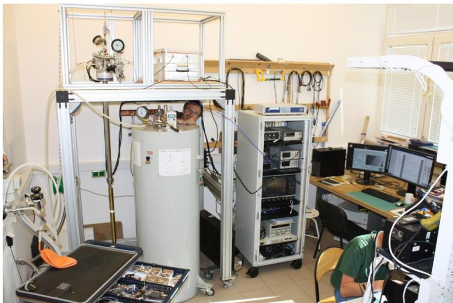
**Fig.19. Heliox laboratory.** Base temperature is 230 mK. The cool-down time from room temperature is only 45 minutes. The holding time for a single experiment with initially full dewar (100l of LHe<sup>4</sup>) is 12 days.
