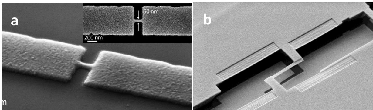
**Fig.3. SEM photos of the nanostructures** routinely obtained in my lab: **(a)** Aluminum nanobridge **(b)** E-beam defined PMMA/MMA mask for Al/Al<sub>x</sub>O<sub>y</sub>/Al tunnel junction (images taken at an angle).
