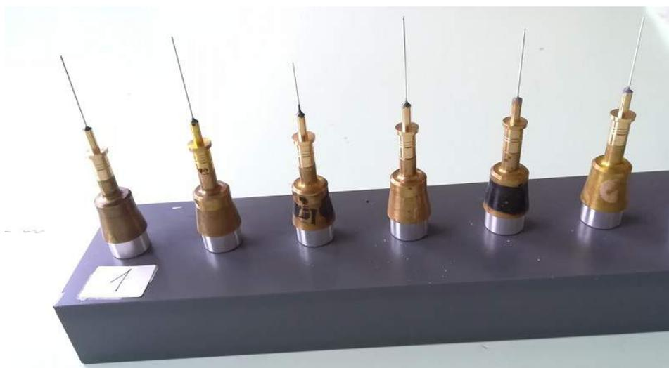
**Figure 3.4:** Photographs of samples prepared for high temperature XRD measurement at synchrotron beamline
