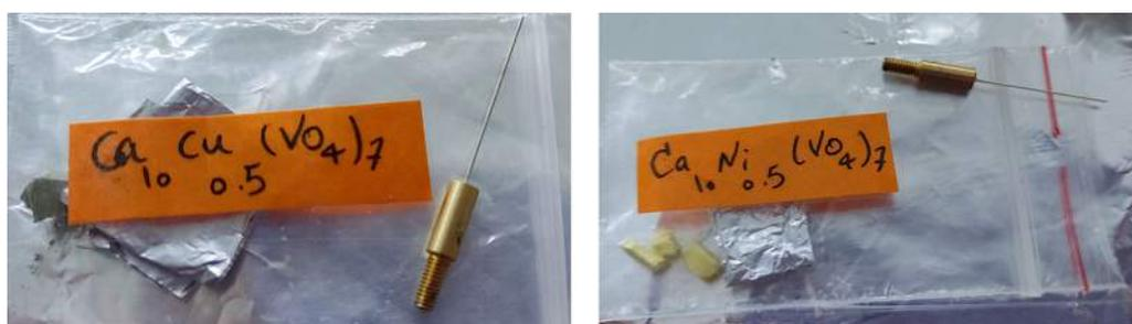
**Figure 3.5:** Photographs of samples prepared for low temperature XRD measurement at synchrotron beamline
