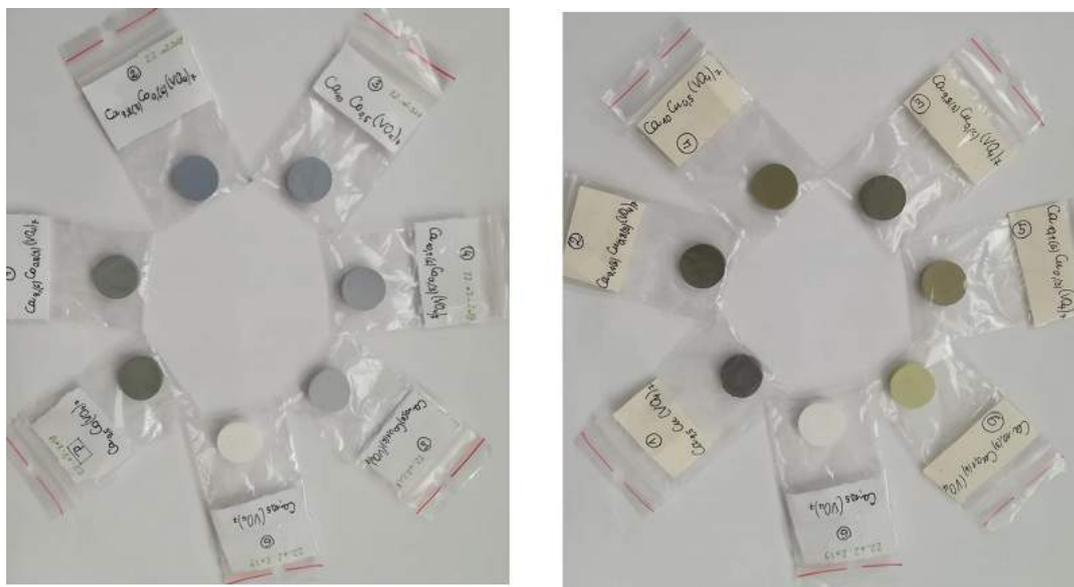
**Figure 3.1:** Photographs of samples synthesised by solid-state reaction (left-  $\text{Ca}_{10.5-x}\text{Co}_x(\text{VO}_4)_7$ , right-  $\text{Ca}_{10.5-x}\text{Cu}_x(\text{VO}_4)_7$ )
