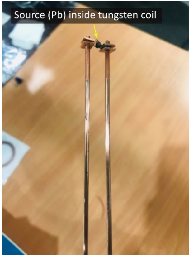
Figure 3.7: Joule heating evaporator system for controlled evaporation of Pb in which a tungsten coil is used to hold Pb.
