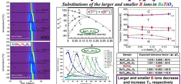
Prediction of increasing  $T_C$  by increase of the  $[\text{B}-\text{O}]$  bond tension was verified. Established the essential parameter for displacive ferroelectricity:  $t_E(x, T) > 1$
