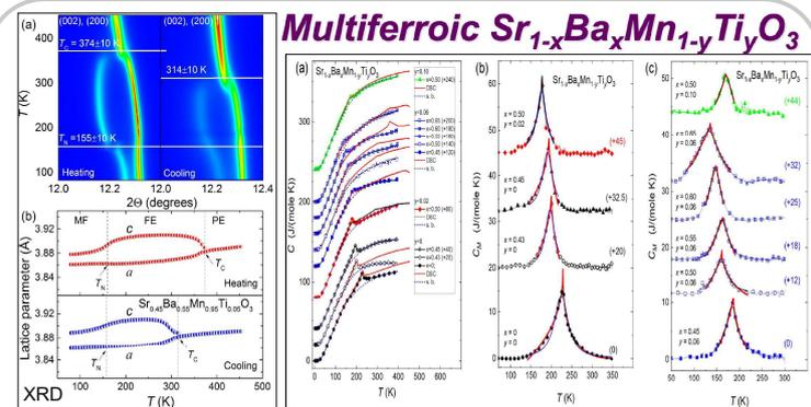
The FE transitions show huge temperature hysteresis at  $T_C$ , an increased  $c/a$  ratio and  $T_C$  to 420 K, as well as reduced suppression of distortion at  $T_N$ . Specific heat studies show that AFM transition changes from the continuous to discontinuous.
