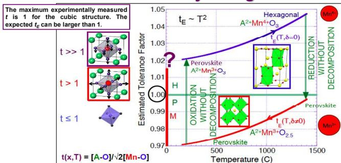
Two-step synthesis was used to remove hexagonal non-FE phase by: Reducing the oxygen content at high temperatures to form perovskite framework by decreasing the tolerance factor below putting back oxygen at low temperature by annealing.
