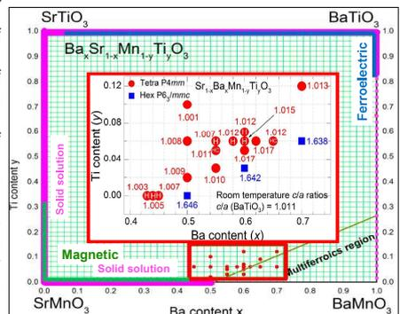
We have achieved the FE distortions in magnetic perovskites  $\text{Sr}_{1-x}\text{Ba}_x\text{Mn}_{1-y}\text{Ti}_y\text{O}_3$  when the Mn-O bonds were stretched beyond equilibrium lengths.
