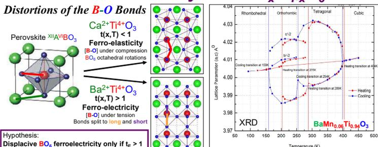
Hypothesis: Displacive  $\text{BO}_6$  ferroelectricity only if  $t_E > 1$
