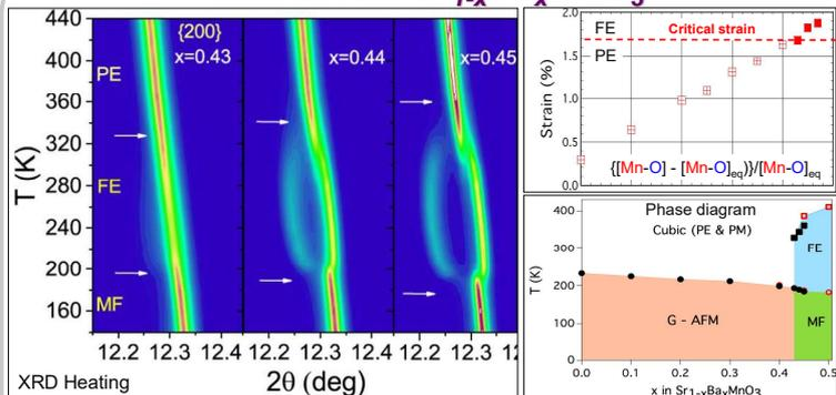
Compositions  $x = 0.43 - 0.45$  show multiferroic properties. The required elongation of the  $[\text{Mn}-\text{O}]$  bond is 1.7% to split it into long and short bonds along the  $c$ -axis.
