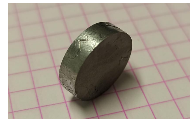
PbTe-CdTe nanocomposite sample cut from an ingot
