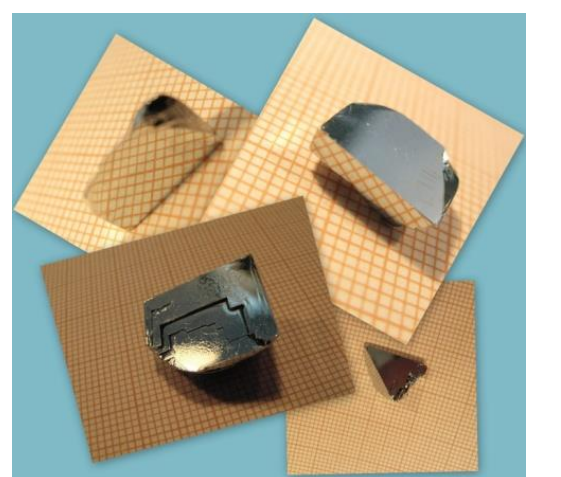
Pb 1-x Cd x Te solid solutions monocrystal with high Cd content obtained by self-selecting vapor growth (SSVG) method [3]
