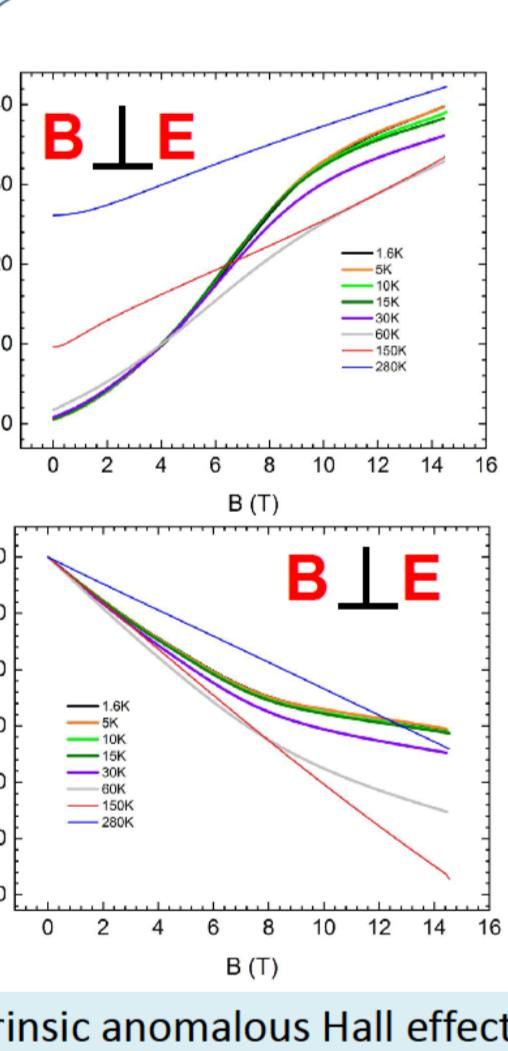
Chiral anomaly observed in  $(\text{PbTe})_{0.6}(\text{SnTe})_{0.4}:\text{Cr}$  in broad temperature range 1.6K to 60K
