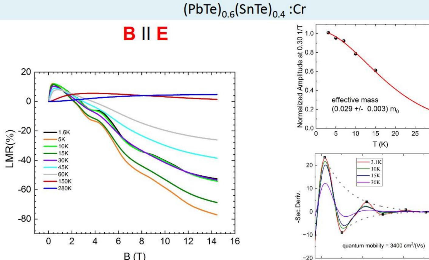
analysis of Shubnikov de Haas oscillations - index plot intercept  $(\text{PbTe})_{0.6}(\text{SnTe})_{0.4}:\text{Cr}$
