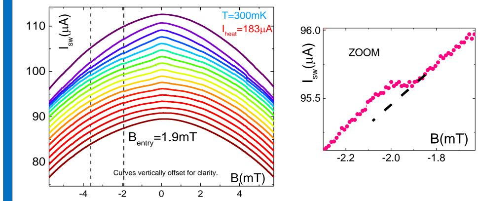
Absorption of QPs by a single vortex is visible as a small enhancement of the switching current observed on the  $I_{sw}(B)$  curves measured at various delays after application of the heating pulse. The kink corresponds exactly to the field where a single vortex entry into the box is expected.
