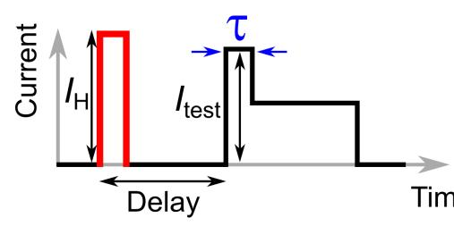
Pump and probe protocol [1-4] is convenient to investigate thermal transients of the nanostructure. We use it to study quasiparticle diffusion in Time vortex state.
