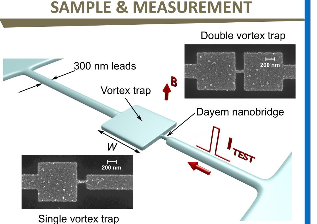
The sample consists of the square vortex trap(s) in immediate contact with a short Dayem nanobridge. The traps are connected to the contact pads via a ~100  $\mu$ m-long and 300-nm wide leads. Electric pulse is applied to one contact pad, while the second pad is grounded. Insets show SEM photos of the typical aluminum structures of the single and double vortex traps.
