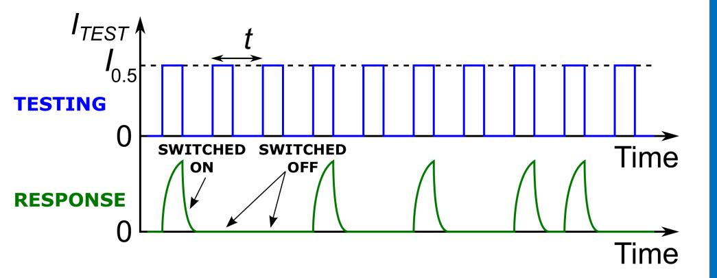
We use the same measurement protocol like in our previous works [1-4]. We send a train of *N* pulses to the nanobridge in order to determine its switching probability *P*. For a certain current amplitude of the testing pulses ( $I_{0.5}$ ) the nanobridge switches to the normal state around *N*/2 times. We call it switching current  $I_{sw}$ .
