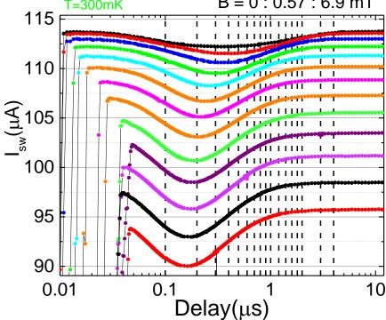
We place a small box on the way between the heater and the detector. We measure diffusive profiles at various magnetic fields.
