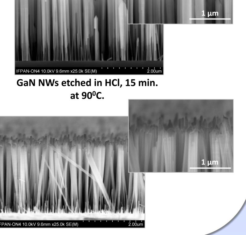
GaN NWs etched in a 10% solution of KOH in water, 40 s at RT.
