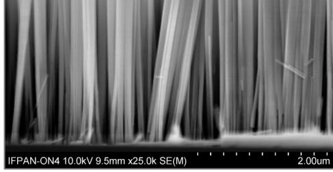
GaN NWs grown by PA MBE on a Si wafer
