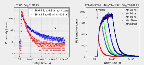
The emission and decay of the PL line of indirect excitons under the condition of their excitation by pulses of different duration. Under-barrier excitation was used.
