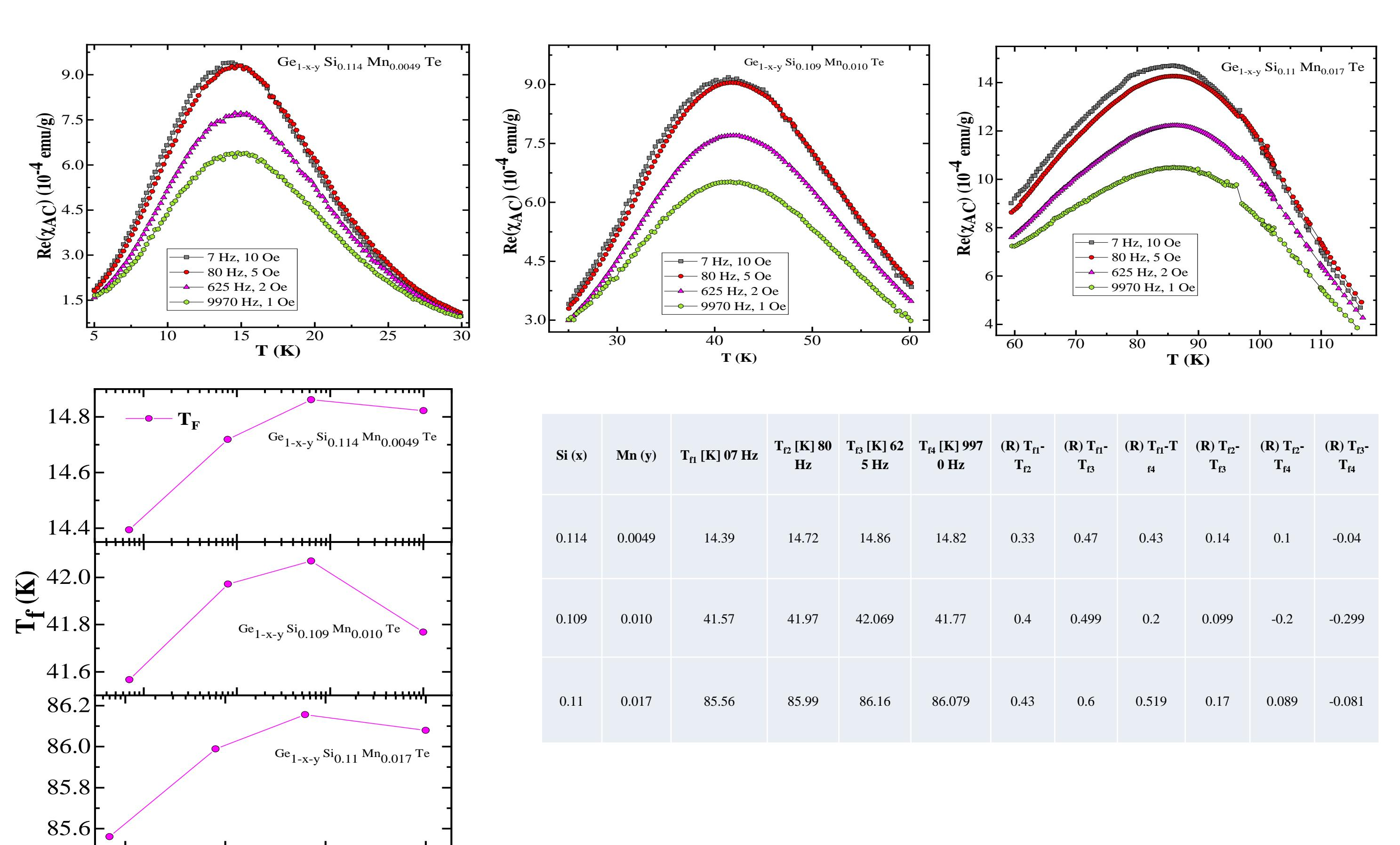
Magnetic susceptibility with temperature measured for different ac magnetic field frequencies and freezing temperature  $T_f$  for different frequencies.
