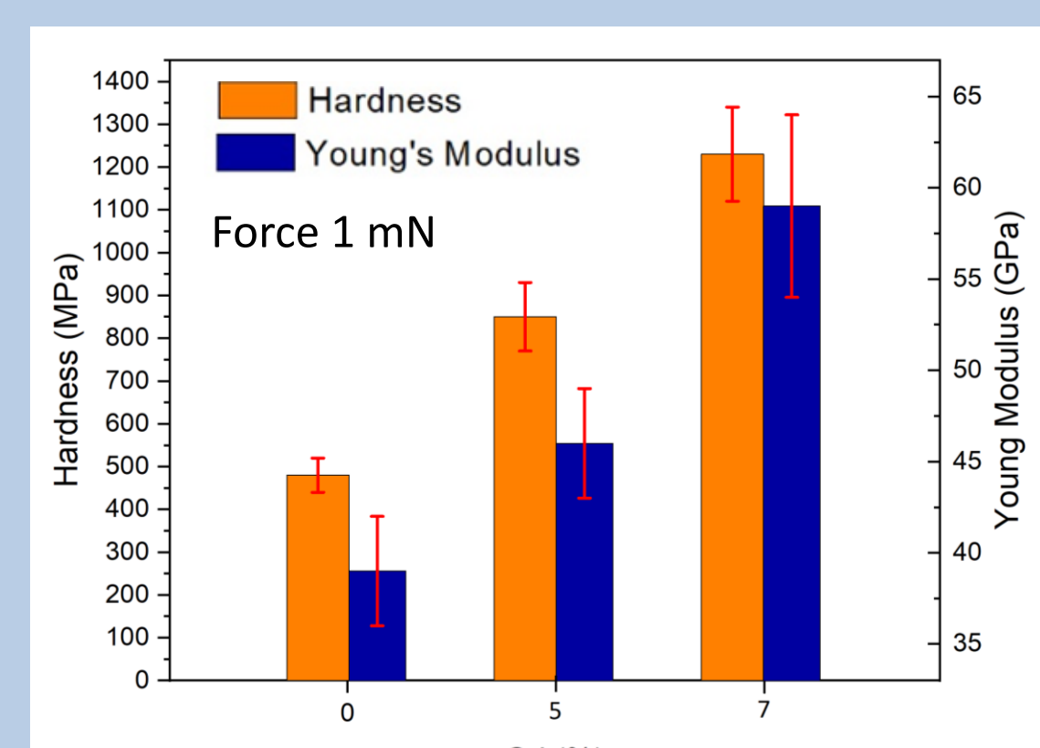
Young modulus and microhardness for (Pb,Cd)Te epitaxial layers as a function of total Cd content.
