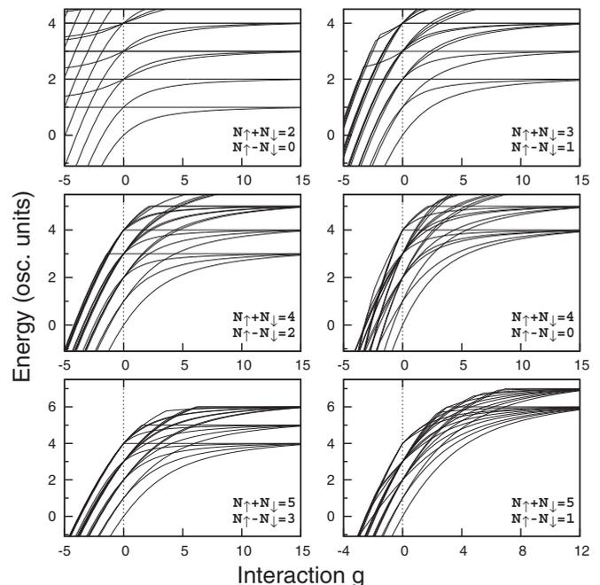
FIG. 1. We plot the energy  $E - E_F$  as a function of the dimensionless interaction strength  $g$  for different combinations of spin-up and spin-down particles. The energy offset  $E_F$  is the Fermi energy of the noninteracting system. We find ground-state degeneracies in the limit of strong interactions. We plot first 20 eigenenergies of the Hamiltonian in Hilbert spaces with fixed  $S_z = N_\uparrow - N_\downarrow$ , but without fixing the total spin.
