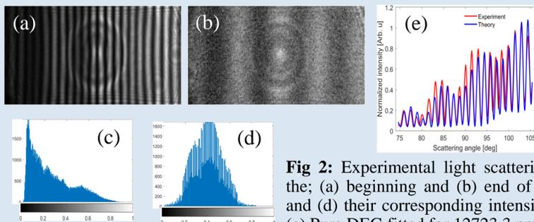
**Fig 2:** Experimental light scattering patterns at the; (a) beginning and (b) end of evolution. (c) and (d) their corresponding intensity histograms. (e) Pure DEG fitted for 12723.3 nm droplet.
