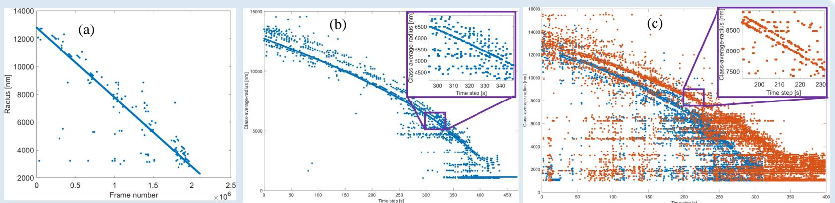
**Fig 4:** Classification of light scattering patterns from microdroplets; (a) theory (b) experiment (pure diethylene glycol) and (c) glycol with polystyrene nanoparticles.
