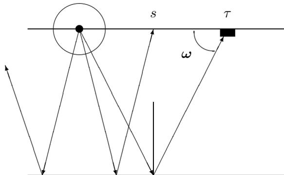
Fig. 2. Schematic view of a path of sound signal reflected from the bottom.
