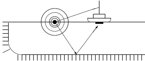
Fig. 1. Schematic view of the way of experimental investigation of a sea-bottom profile.
