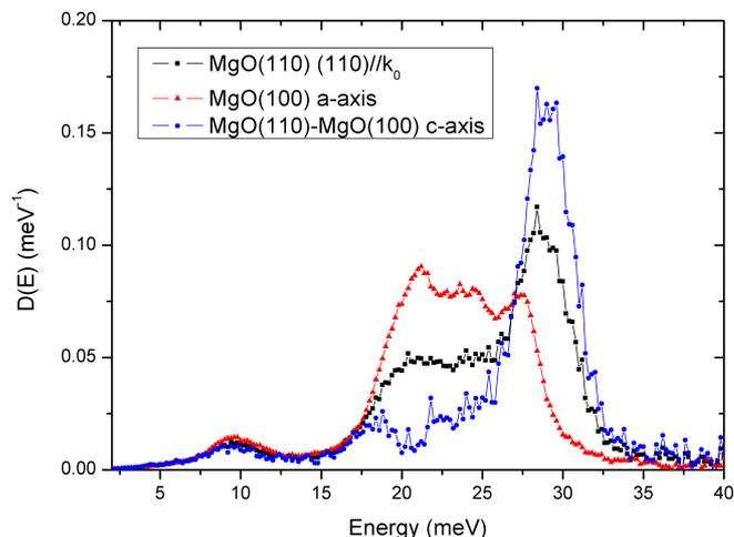
Fig. 2: Phonon density of state of the FePt along the different crystalline axis, extracted from the NIS spectra. Notice the high anisotropy between the a- and c-axis PDOS.
