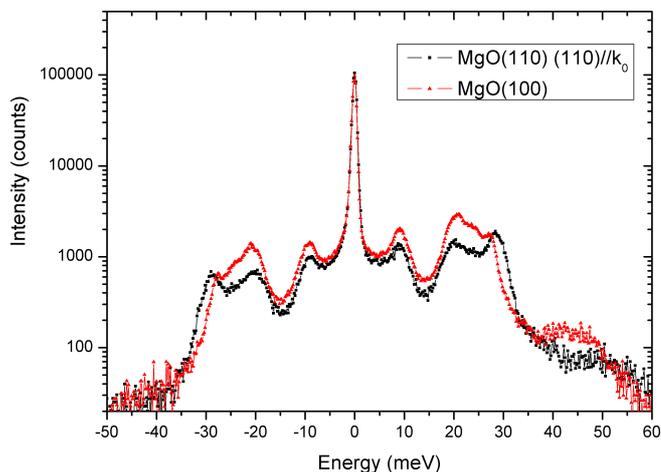
Fig. 1: Nuclear inelastic spectra recorded with 0.8 meV resolution on 30 nm FePt grown on MgO(100) and MgO(110) substrates.
