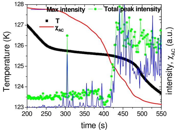
Fig. 3. Time profile of temperature, AC susceptibility and the intensity of  $(1\ 1\frac{1}{2}\ 2)$  superlattice peak of “553” sample at the Verwey transition
