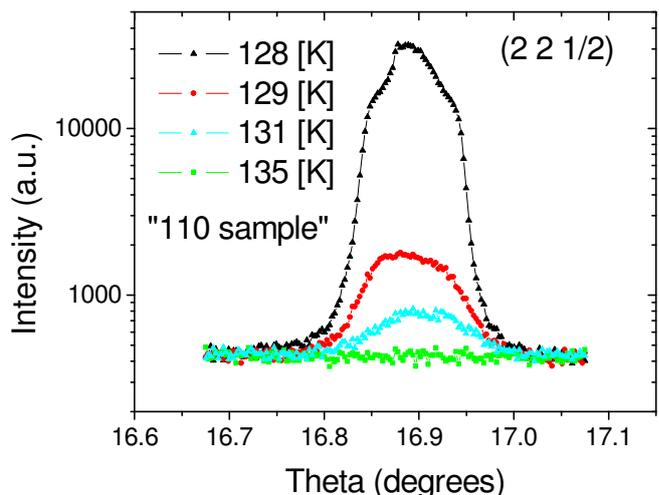
Fig. 2. Temperature dependence of part of superlattice peak Q-scan of just above the transition for “110 sample”
