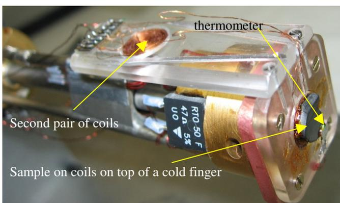
Fig. 1. The sample on top of AC susceptibility setup (attached to the cryostat cold finger) and with Pt1000 thermometer
