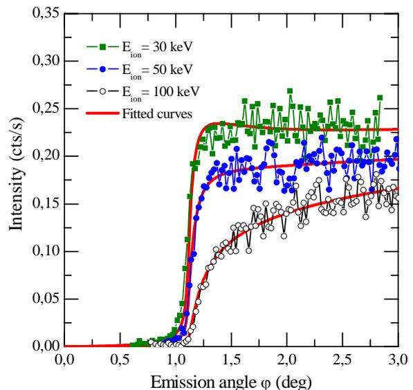
Measured intensities of the Al-K $\alpha$  fluorescence line excited by 1570 eV photons versus the grazing emission angle for the Si wafers implanted by Al ions for different ions energy.
