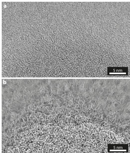
**Fig. 1** Comparison of conventional TEM imaging and EWR phase imaging. (a) near focus TEM, and (b) EWR phase.
