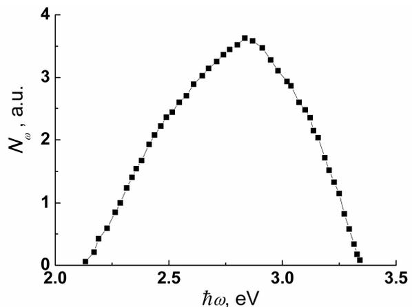
Fig. 1. Photoluminescence spectra of TiN thin films, measured at 300 K
