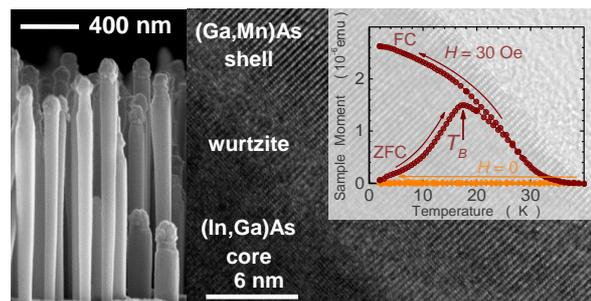
**Figure 1.** Electron microscopy images: left panel - SEM, right panel - high resolution TEM; of Au-catalysed (In,Ga)As-(Ga,Mn)As core-shell nanowires. The inset to the right panel shows temperature dependent magnetic moment of the NWs embedded in the PMMA resist and separated from the growth substrate.
