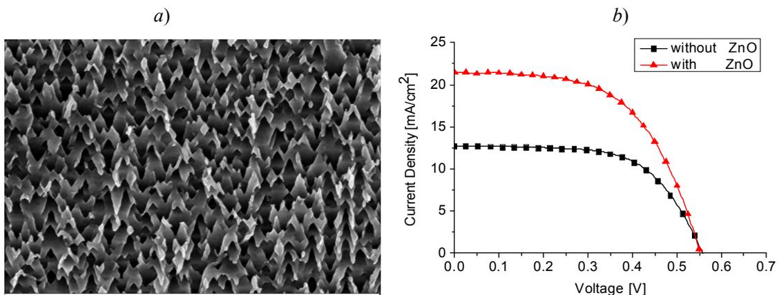
Figure 1: a) SEM image textured surface of ZnTe, b) Illuminated current–voltage characteristics for n-CdTe/p-ZnTe heterojunctions with and without ARC.
