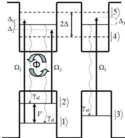
**Fig.1** Structure consisting of double tunneling-coupled quantum wells. Here  $\Delta_1$ ,  $\Delta_2$  are laser detunings of optical fields,  $\Omega_1$ ,  $\Omega_2$ ,  $\Omega_3$  are Rabi frequencies of optical fields and  $V$  is Rabi frequency of low-frequency field,  $2\Delta$  is tunneling splitting.
