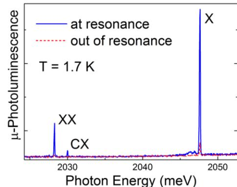
Figure 1. The  $\mu$ -PL spectra of a single CdSe/ZnCdSe QD excited at resonance and out of resonance.
