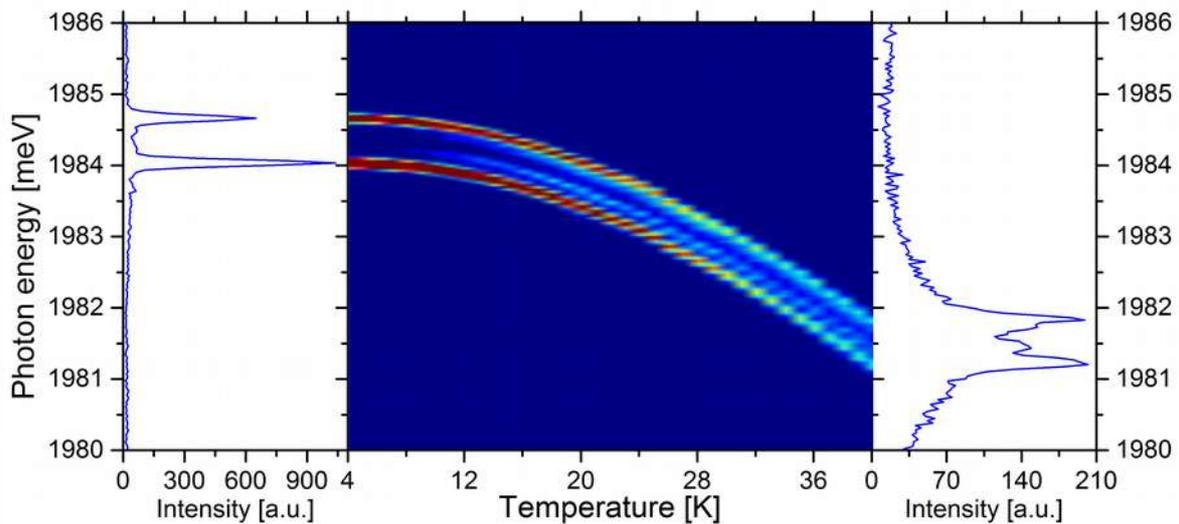
Fig. 1. Map of photoluminescence intensity of neutral exciton line for increasing temperatures.
