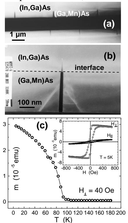
**Fig. 1.** (a), (b) – cross-sectional TEM images of (Ga,Mn)As/(In,Ga)As interface with micro-cracks; (c) temperature (main panel) and field dependence (inset) of the magnetic moment of the same sample (0.3  $\mu\text{m}$  thick  $\text{Ga}_{0.94}\text{Mn}_{0.06}\text{As}/\text{In}_{0.20}\text{Ga}_{0.80}\text{As}$ ).
