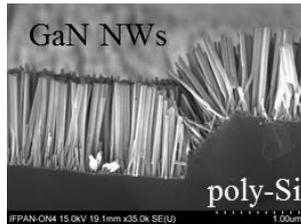
Fig.1. SEM image of GaN NWs grown on mc-Si substrate.
