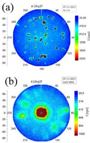
Fig.2. X-ray diffraction 111Si (a) and 0002GaN (b) pole figures of GaN NWs on mc-Si.
