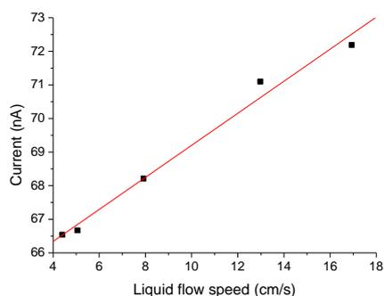
Fig. 1 Relationship between liquid flow speed and generated current signal.
