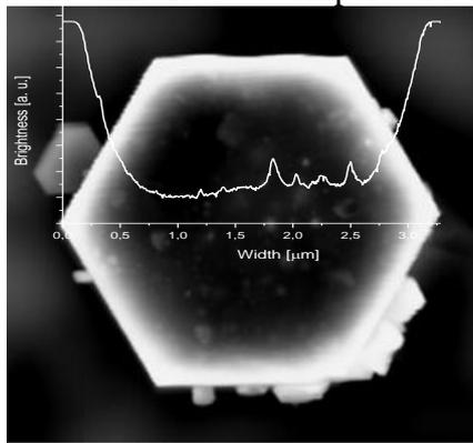
Fig. 1. CL map of the upper surface of ZnO nanorod obtained from solution of pH=7.
