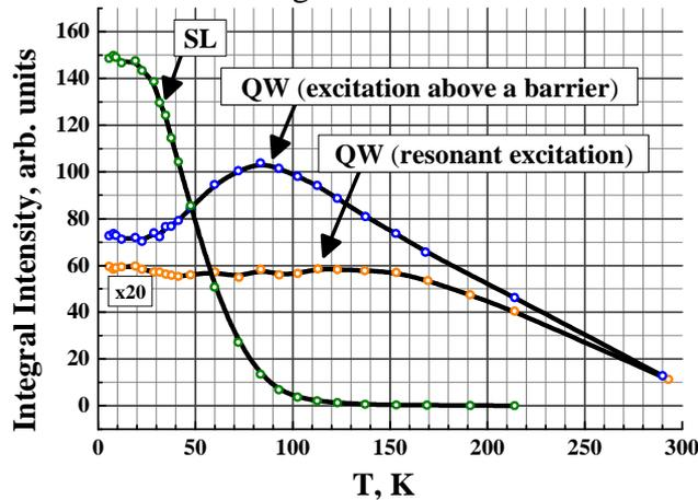
Fig. 1. Temperature dependence of integral intensity of PL in the SL and enlarged QW under resonant excitation and excitation above the SL band-gap.
