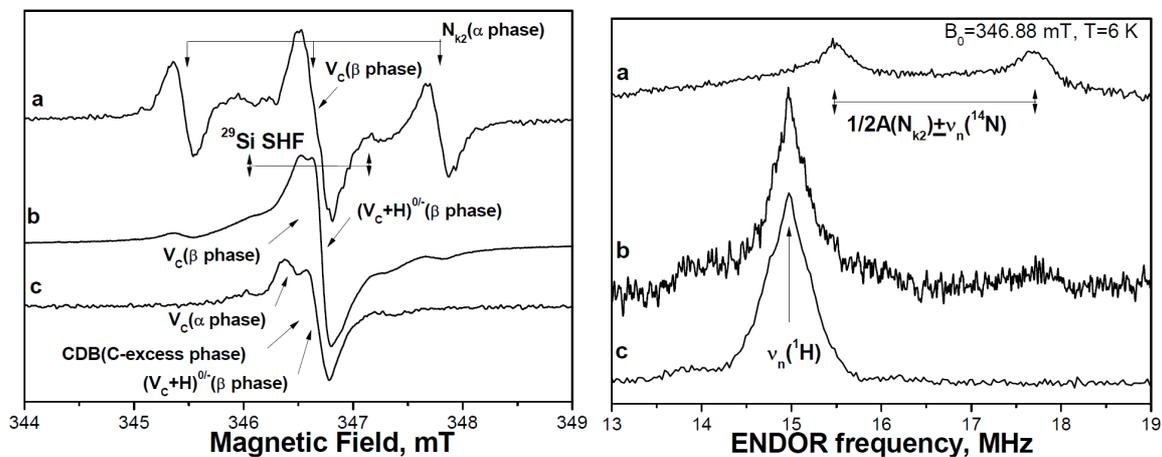
**Fig. 1.** The X-band first derivative of FS ESE (a) and pulsed ENDOR (b) spectra measured in np- and mp-SiC with  $R > 100$  nm (a),  $50 \text{ nm} < R < 100$  nm (b),  $R < 50$  nm (c) at  $T = 6$  K.
