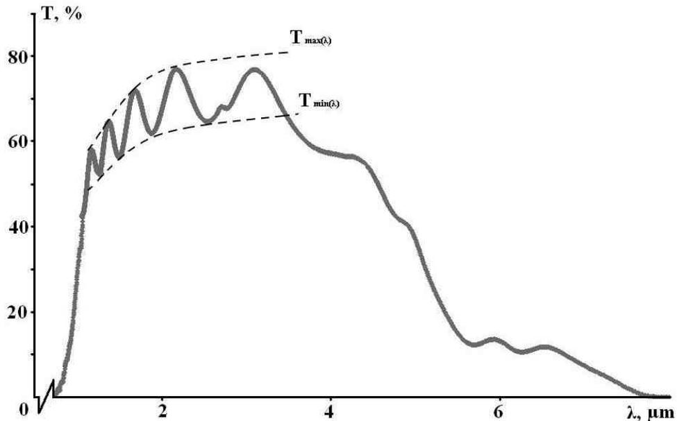
Fig. 1. Dependency of transmission coefficient on wavelength of electromagnetic radiation at  $T = 300$  K for thin film  $\text{Cu}_2\text{ZnSnS}_2\text{Se}_2$
