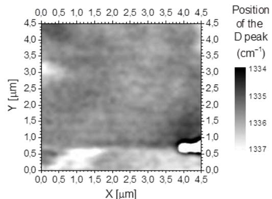
Figure 2. Map of D peak position in graphene Raman spectrum with visible distribution reproducing NWs surface density.
