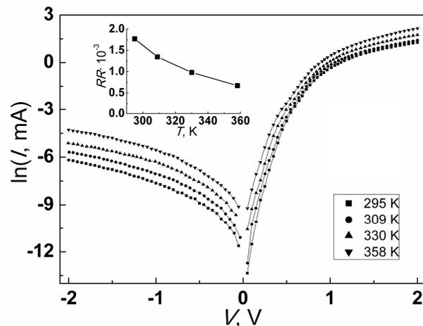
Fig. 1. I-V characteristics of the n-TiN/p-CdZnTe heterojunctions at different temperatures. The inset shows the temperature dependence of the rectification ratio.
