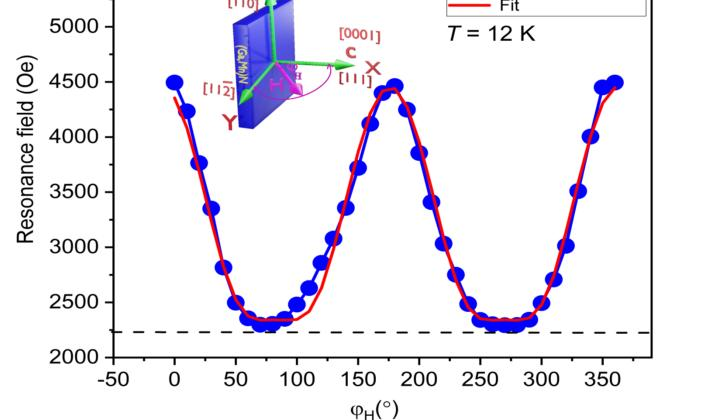
Figure 6: Angular dependence of the ferromagnetic resonance fields for the magnetic field rotating within the  $[1\overline{1}0]$  plane.
