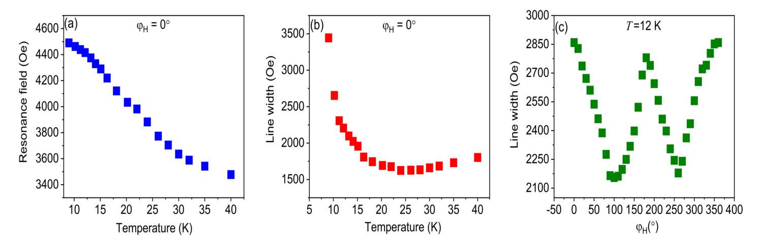
Figure 7: (a) Temperature dependence of the resonance field for the magnetic field along the out of plane [111] direction. (b) Temperature dependence of the line width for the magnetic field along the out of plane [111] direction.
