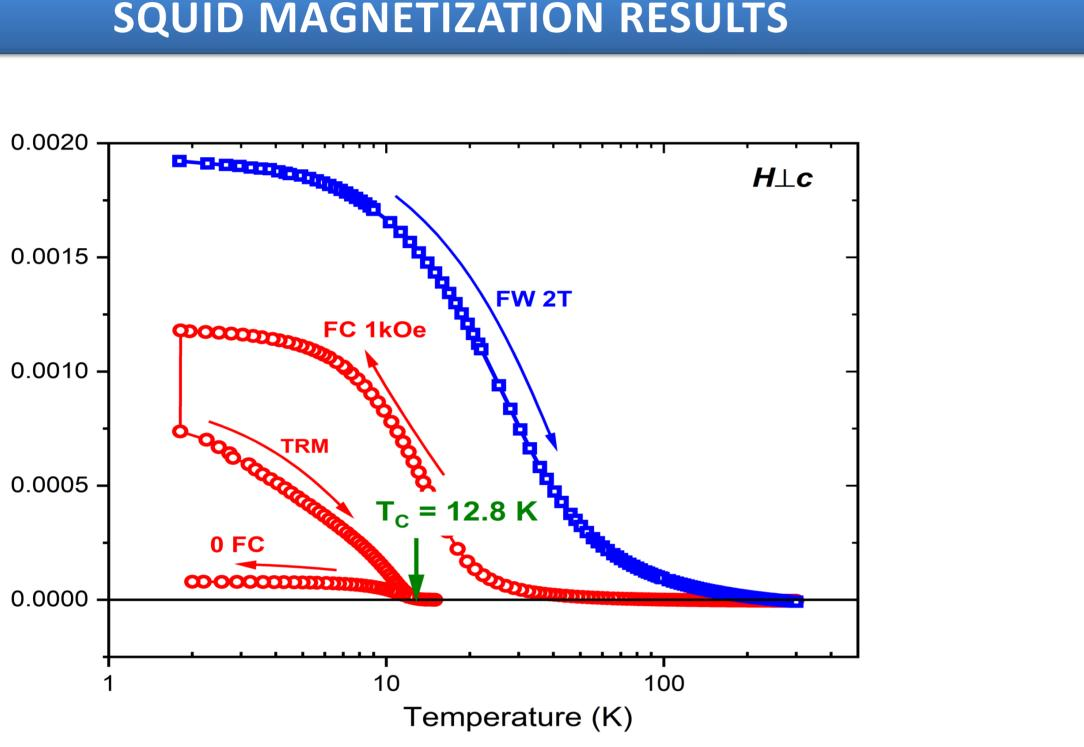
Figure 1: Temperature dependence of the magnetization of (Ga,Mn)N with 9.7% Mn. The sample is initially field-cooled (FC) in a magnetic field of H = 1 kOe and after quenching the field, the thermoremanent magnetization (TRM) is recorded during warming . The temperature at which TRM vanishes indicates the Curie temperature  $(T_c)$ .
