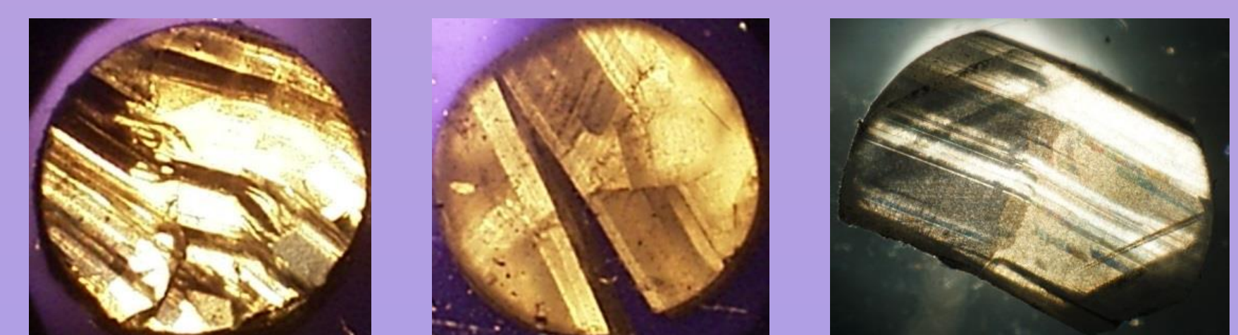
Twinning visible in polarized light of \text{Ga}_2\text{O}_3 cross-section for subsequent crystals
