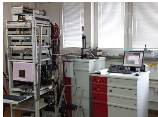
Fig. 1. Two MPMS SQUID magnetometers from Quantum Design. The left one is wired up for electrical-gating experiment.
