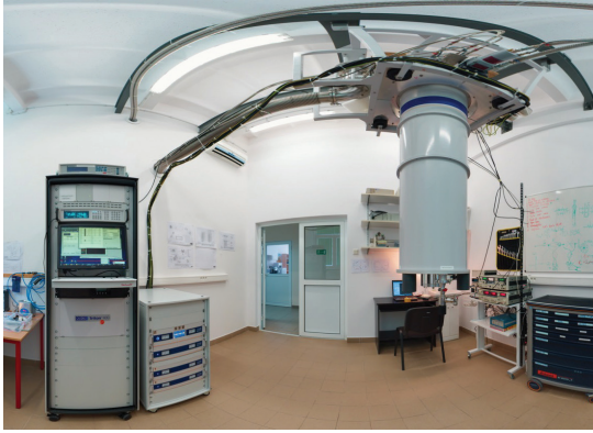
Fig. 3. Triton 400 laboratory. Cryogen-free dilution refrigerator from Oxford Instruments. Samples are cooled to the base temperature of 10 mK in 12 hours with the bottom loading mechanism. Equipped with 6-1-1T vector magnet.
