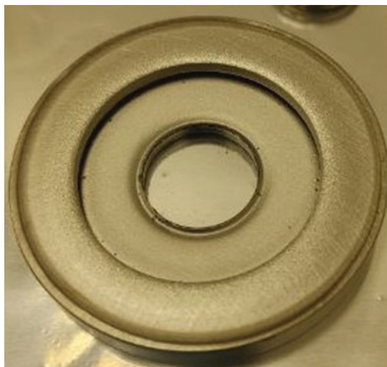
Figure: 2" target with a visible narrow and uneven erosion track, indicating that the flux was not constant during deposition (upper). After source modification (lower panel), the surface was flat after several sputtering processes, meaning that the material was consumed evenly (after [1]).
